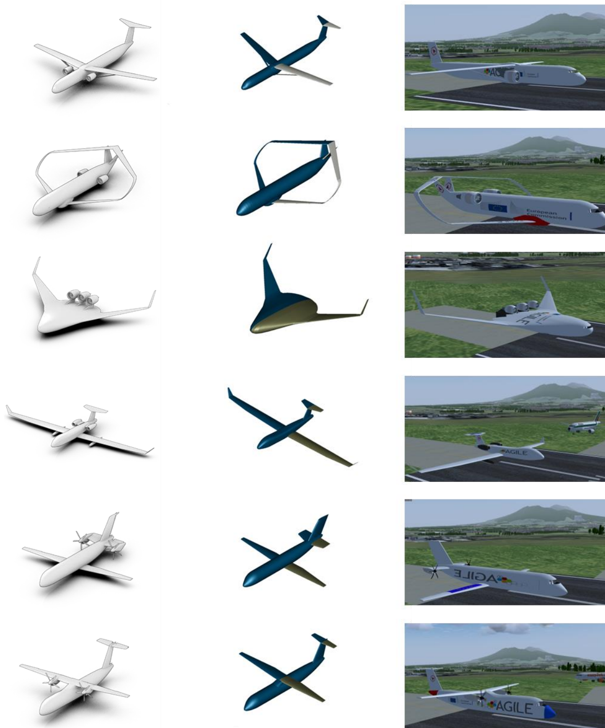
Figure 2 AGILE Novel configurations (left) available in the database and corresponding CPACS models (middle) and FlightGear models (right).
